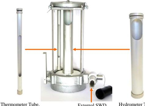
External SWD Fitting. Part No. 60072331212 or 6007233213 Hydrometer Tube. Part No. 6007233166.
